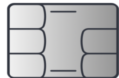
C4 Removed C8 Removed
